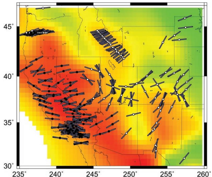
**Fig. 2.** Map of available splitting observations (14, 20, 21) superimposed on mantle shear velocity at a depth of 150 km (10). Circles give station locations. Bar orientations give splitting fast polarization direction  $\phi$ , which equals  $\pm \hat{V}_s$ . We use data only from “red” (slow) areas (solid circles), where the influence of lithosphere on anisotropy is expected to be small.
